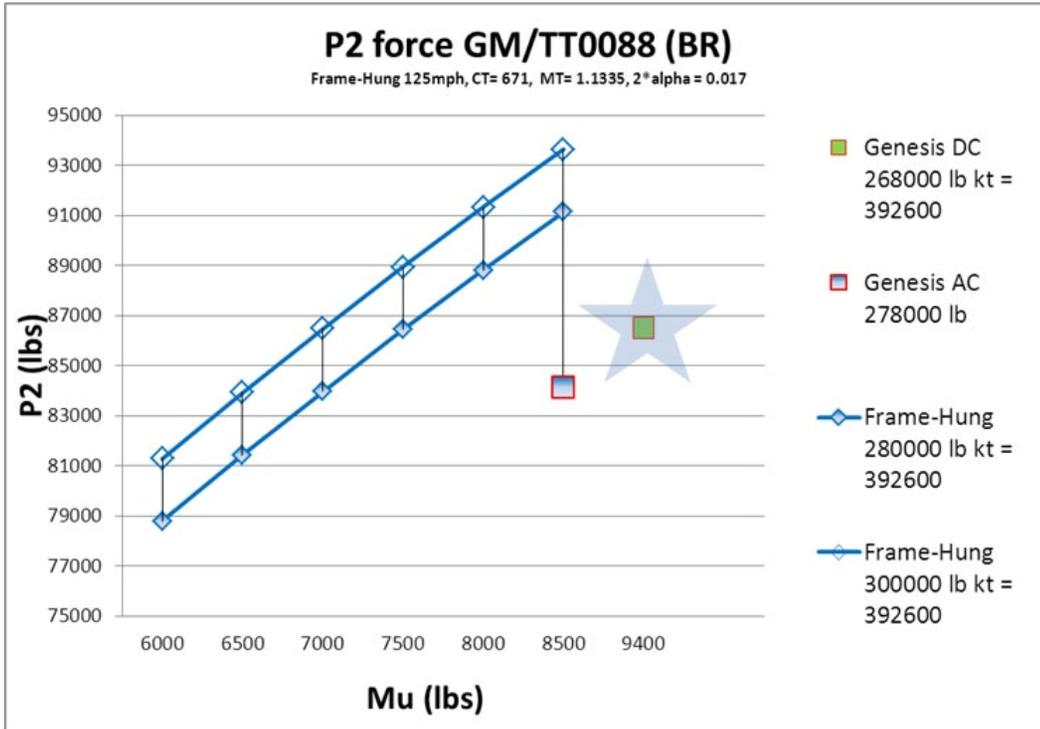
**DC loco** has heavier motor and **higher P2 force** even though the overall locomotive weight is lower
