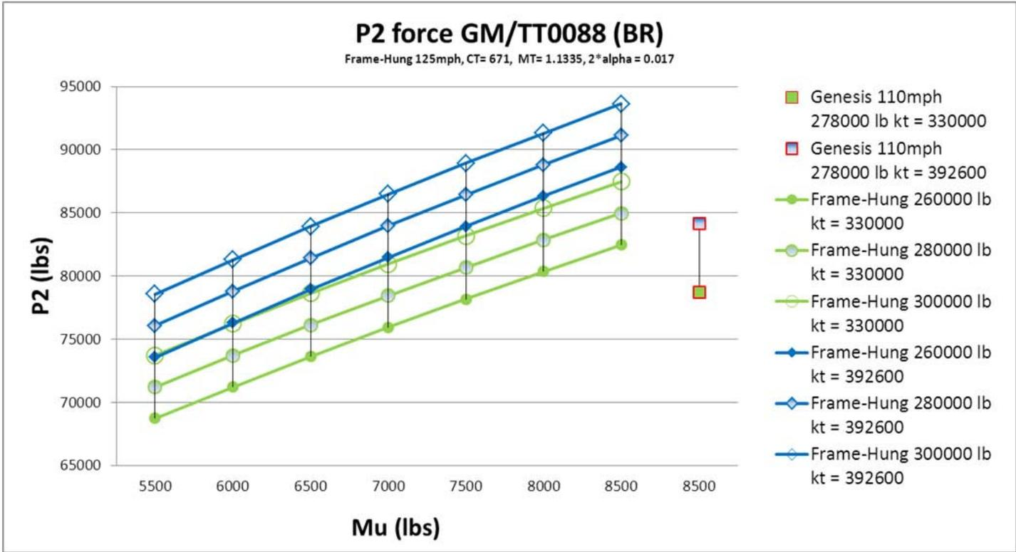
For 300K loco, with Kt= 330,000 we had allowable unsprung weight at slightly above **7,000 lbs.** Changing the Kt to 392,600 drives the allowable Mu to **6000 lbs.**
