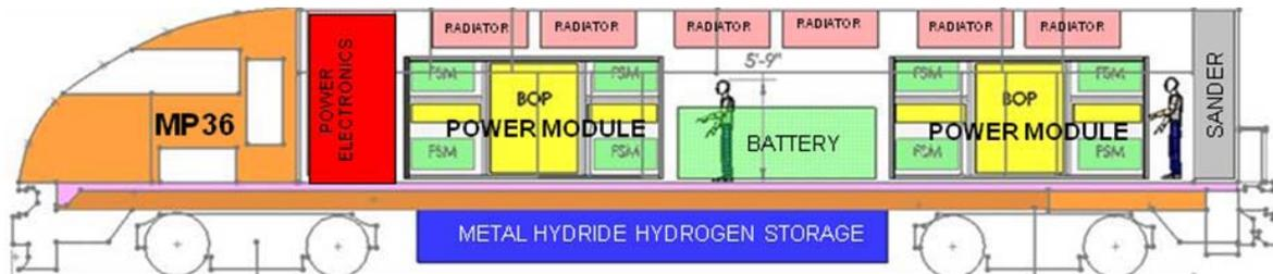
Figure 3: Motive Power MP36 fuel cell powered commuter locomotive concept
