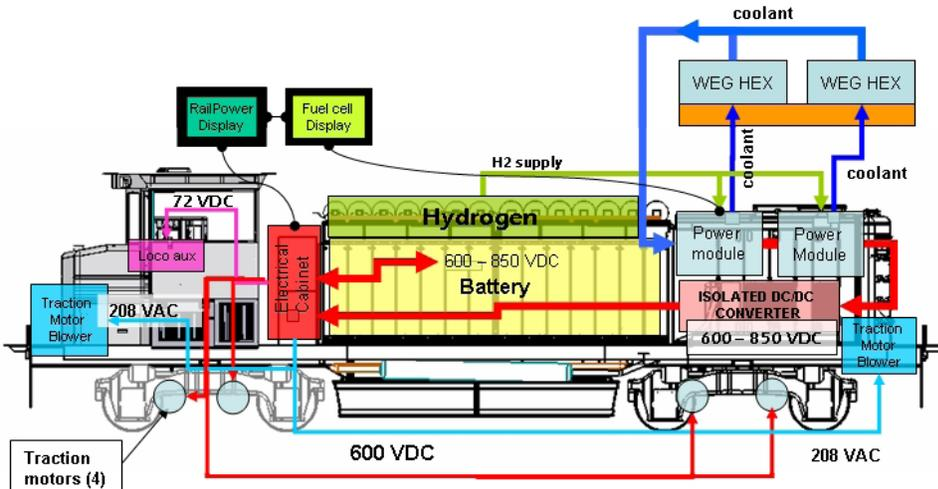
Figure 2: System layout of the fuel cell hybrid locomotive including 250 kW net fuel cell power plant, DC-to-DC converter, hydrogen storage and control interface
