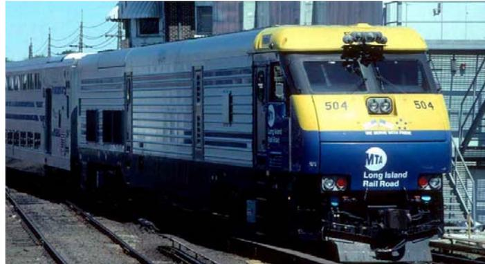
**Vehicle/Technology:** Diesel/3<sup>rd</sup> Rail Line Haul Passenger Locomotive
