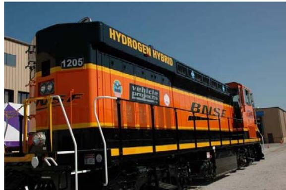
**Figure 1: Fuel cell battery hybrid switcher locomotive**
